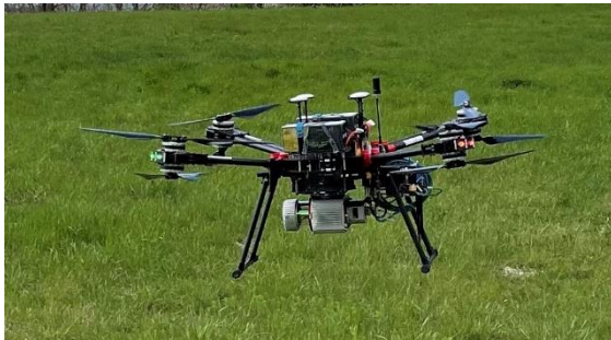
Figure 11: UAV-system equipped with LiDAR, capable of simultaneously carrying several other sensor suites.
